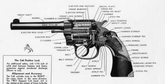
crane against the frame. Proper alignment of chamber and barrel is assured another factor in Colt's Designed Accuracy.
